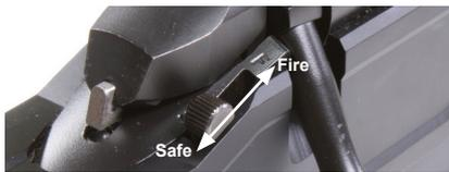
All Bergara Premier rifles and most Bergara Custom rifles utilize a manual safety with a lever located on the right side of the receiver at the rear of the bolt. This lever rocks rearward to the "safe" position and forward to the "fire" position. The rifle's bolt can normally be manipulated while in either position. Some custom triggers or bolt sleeves may feature a safety with a third position that locks the bolt.
